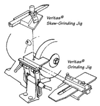
Rest so that there is no more than 1/8" of clearance between the table and the grinding wheel. Don't adjust the table when the grinder is running.
