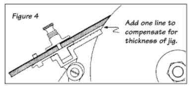
Simply remember to add one line thickness after you have determined where the Angle-Setting Gauge should touch the wheel (Figure 4).
